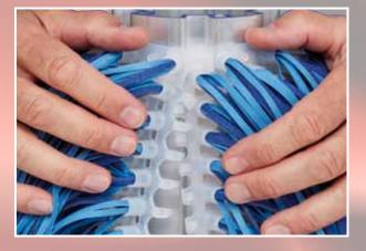
**ProMicro** rail (Keder) quick change system for two-ply washing material
